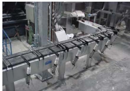
5 Insulated covers with a pneumatic lifting system.
