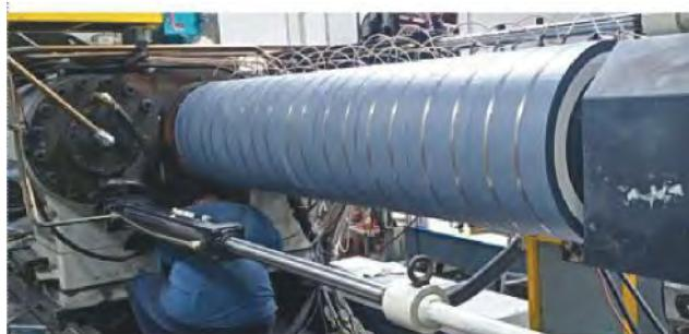
TCS heater bands from Rex Material embed heating elements within an insulated material just 1 in. from the barrel exterior.
